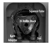
Remove the existing squeeze tube (black tube with lubricant), complete with the two black barb adaptors and tube nuts on the bottom, by gently pulling the left side tube barb adaptor towards you and lifting from left to right. Scan the QR code below to see our video instructions and further detail.
